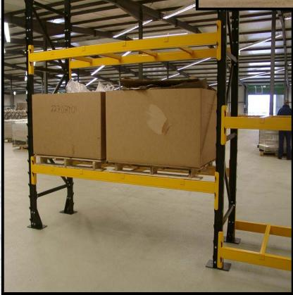
Standard platform takes 6000lbs per pair of beams (uniformly distributed)
